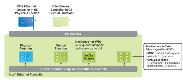
Figure 1. Overview of Intel® Virtualization Technology for Connectivity
