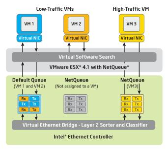
Figure 2. Virtual Machine Device Queues
