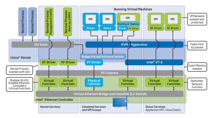
Figure 5. Port Partitioning in a combined bare-metal Linux\* and virtualized environment
