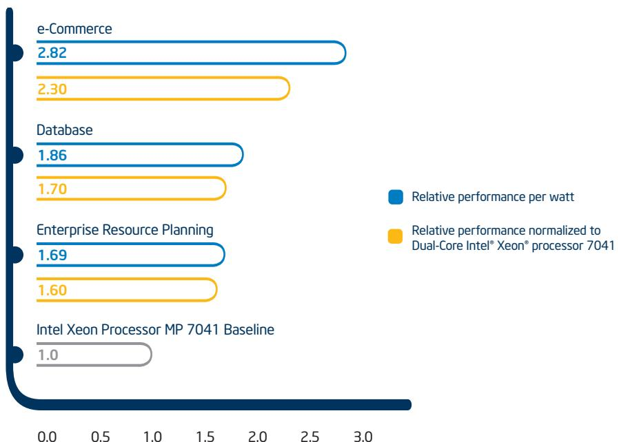
**Dual-Core Intel® Xeon® processor MP 7140M (3.40 GHz, 16 MB L3) processor scaling**
