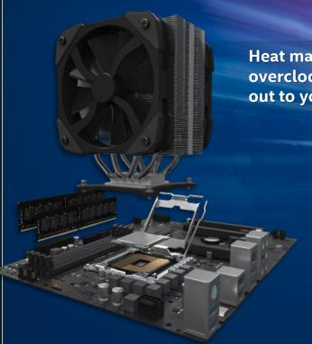
Heat management is critical for any successful overclock. STIM helps maximize heat transfer out to your cooling solution.
