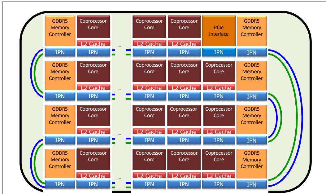
Figure 2-4. Intel® Xeon Phi™ Coprocessor Silicon Layout
