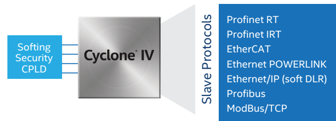
Figure 6. Security CPLD Enables License for Selected Ethernet IP
