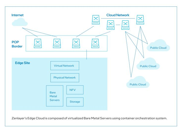
The solution is part of an Ethernet Virtual Private Network (EVPN) for multi-tenant isolation. The Zenlayer Edge Cloud is composed of bare metal servers, VMs, and containers, and offers premium services with high density computing capacity, high performance storage, ultra-low network latency to local regions, and can also enable service integrations with public clouds.
