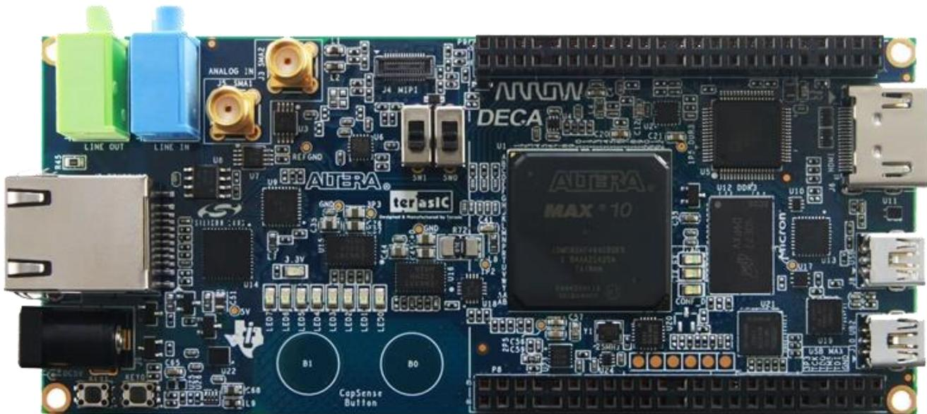
There are many components on the DECA board including the LEDs, CapSense Buttons, USB, Ethernet, HDMI and MIPI Interfaces. There is a gesture sensor on the back of the board and an Audio Line In/Out jack on the top.
