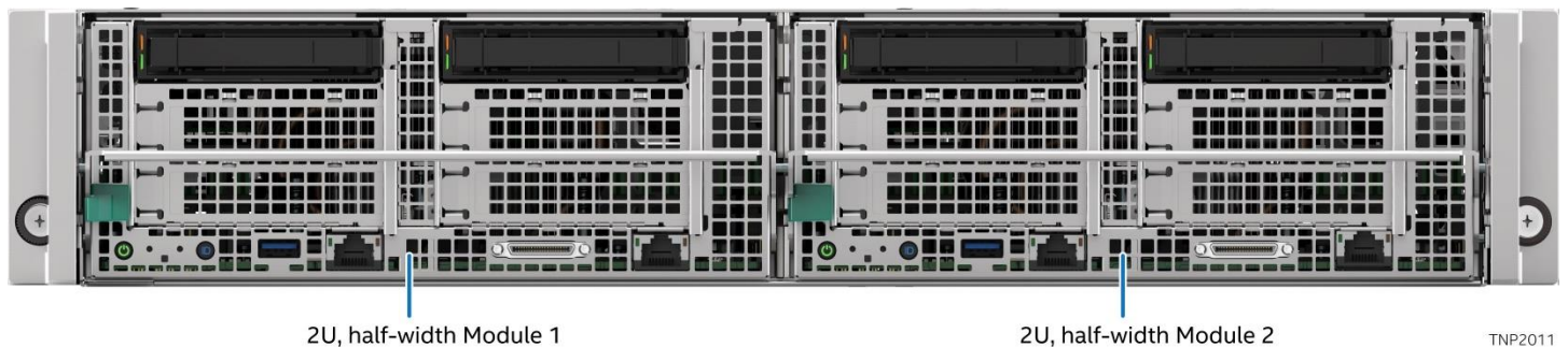
Figure 106. Module Identification for Two-Module System Configuration
