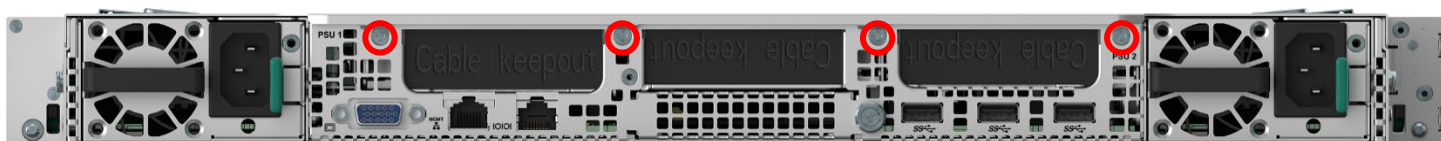
Figure 20. Rear Panel Shipping Screw Holes
