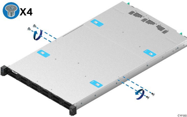
Figure 16. System Top Cover Shipping Screws
