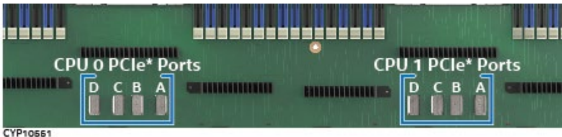
Figure 76. PCIe* SlimSAS* Connectors
