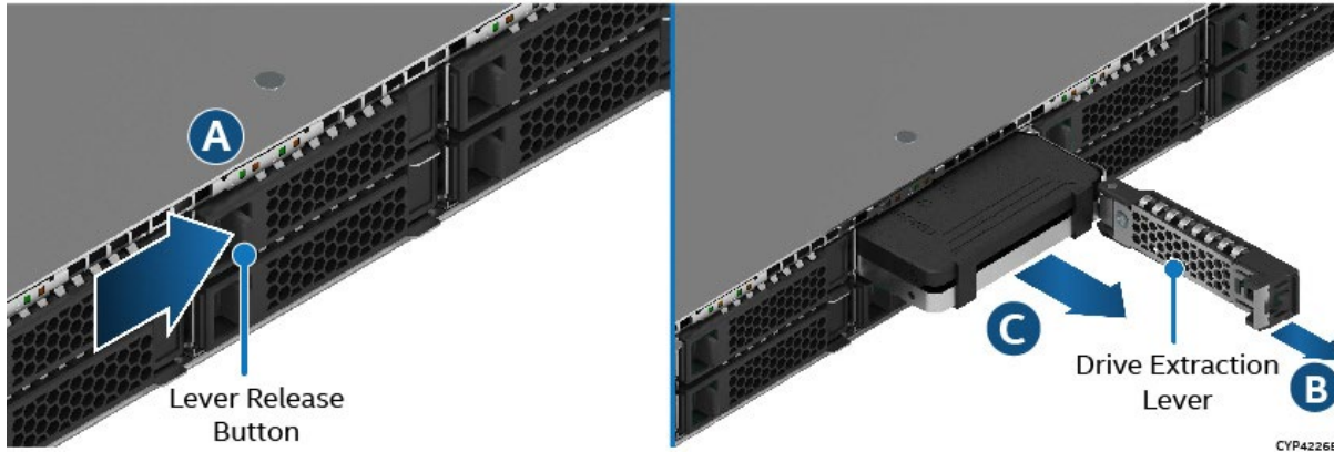
Figure 64. 7 mm Drive Removal from 2.5" Drive Bay
