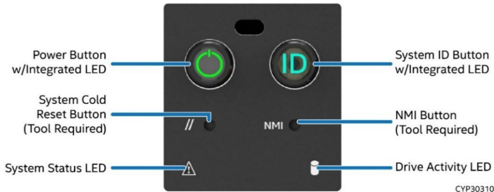
Figure 91. Front Control Panel Features
