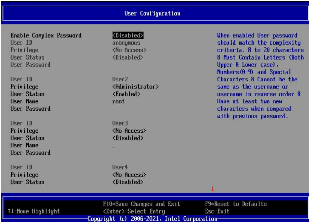
Figure 10. BIOS Setup User Configuration Screen
