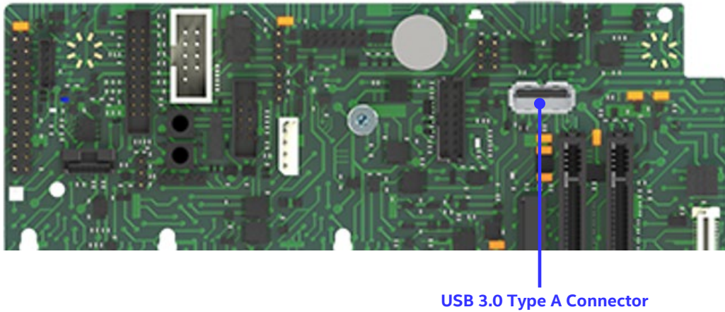
Figure 43. Internal USB 3.0 Type A connector
