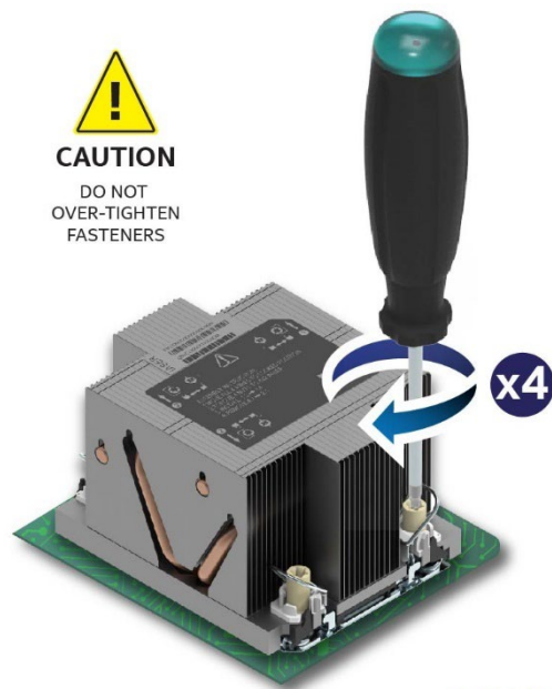
Figure 72. Tighten Heat Sink Fasteners
