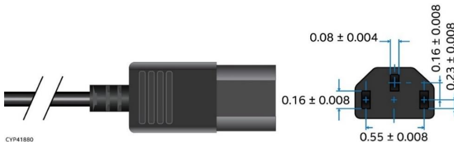
Figure 22. AC Power Cord Specification
