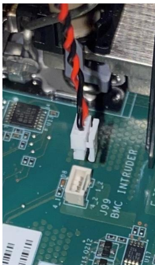
Figure 12. Chassis Intrusion Switch Cable to Server Board
