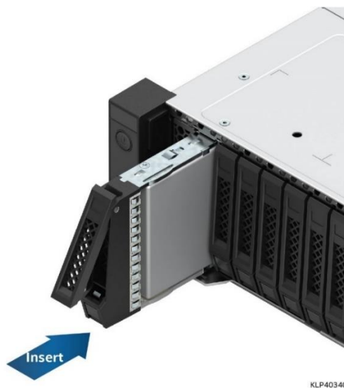
Figure 87. Drive Assembly Installation to Front Drive Bay
