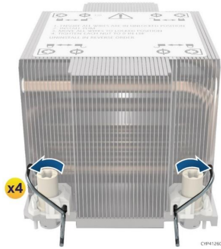
Figure 102. Processor Heat Sink Anti-tilt Wires in the Outward Position
