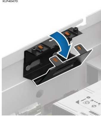
Open bracket to install cables
