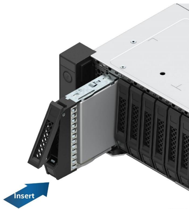
Figure 49. Installation of Drive Assembly to Front Drive Bay
