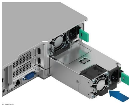
Figure 82. Power Supply Module Installation
