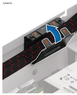
Cables routed and secured
