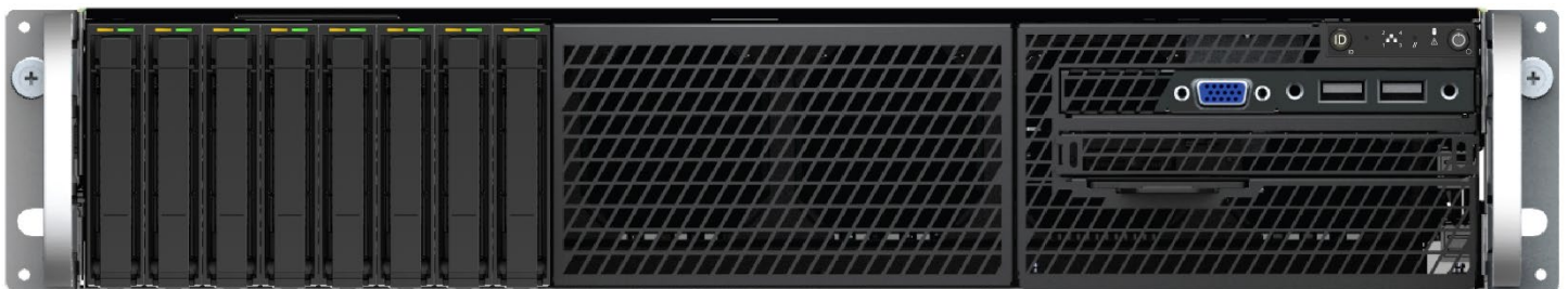
Figure 120. 8 x 2.5" Drive Bay Configuration (Intel® Server System R2208WF...)
