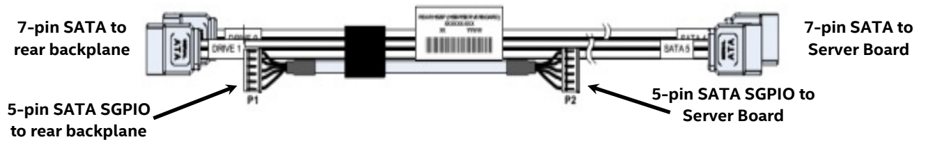
Figure 99. Rear HSBP SATA & SGPIO Cable Bundle
