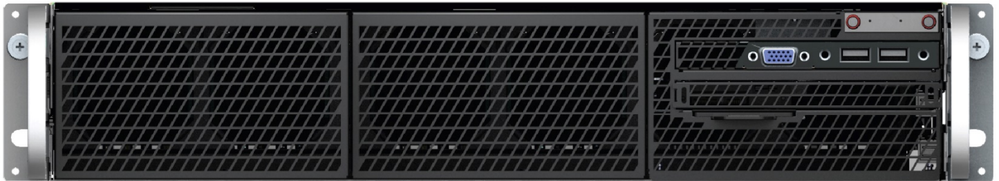
Figure 1. Intel® Server Chassis R2000WFxxx – No Installed Front Drive Accessory Kit Options
