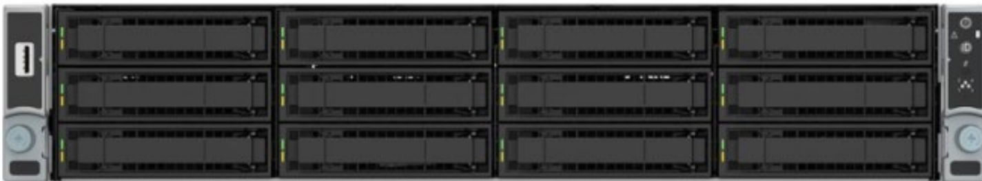
Figure 2. Intel® Server Chassis R2312WFxxx – 12 x 3.5" Front Drive Bay
