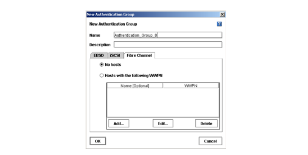
Figure 165. Creating Fibre Channel Access in New Authentication Group
