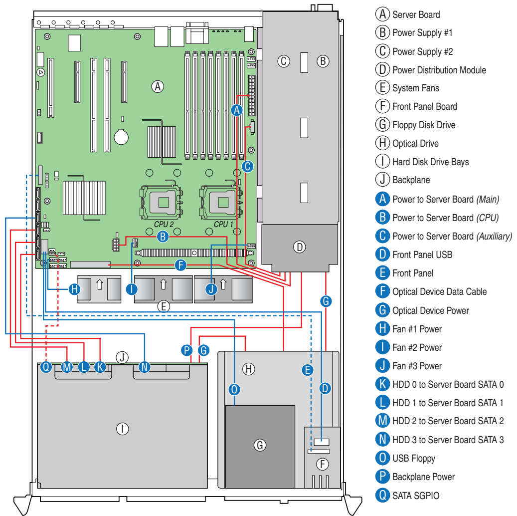
Figure 58. Cable Routing (SR2520SAX/SR2520SAXS and SR2520SAXR/SR2520SAXSR)
