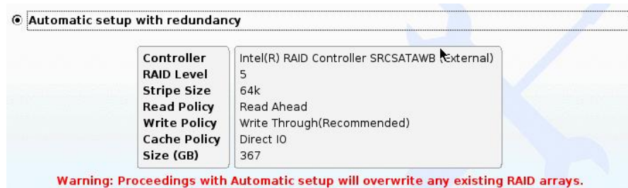
Figure 3-29: Automatic Setup RAID with Redundancy
