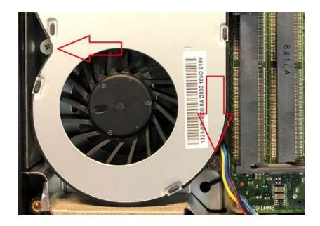
4. Place the black tape back down onto the fan assembly.
