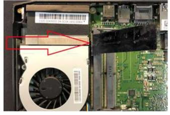
4. Remove the two screws that secure the fan assembly to the heatsink.
