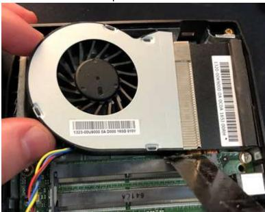
3. Secure the fan to the heatsink with the two screws.
