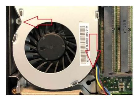
5. To remove the fan, lift the circular fan hub while pulling the fan towards you. There may be some resistance from the black tape on the underside of the fan - this is normal - a little wiggling from side to side may help.
