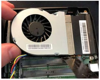
Warning! Don't remove the heat sink from the motherboard.
