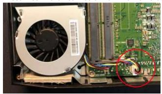
3. Peel back the black tape from the top of the fan assembly towards the memory slots. Do not completely remove the tape.
