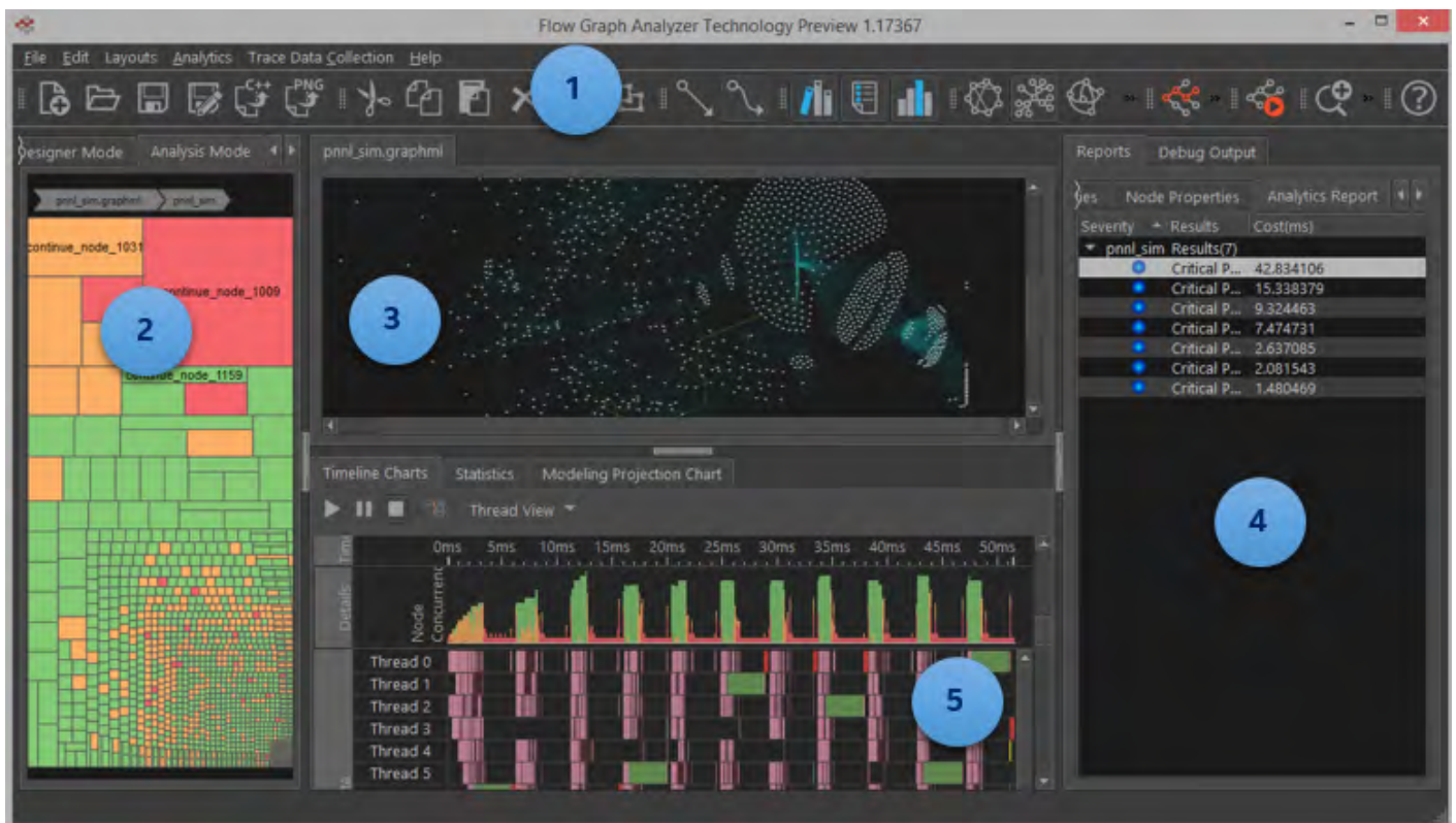
4 Intel FGA showing a captured graph and associated trace data
