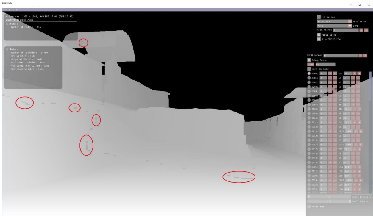
Figure 9: Silhouette bleed-through in a well-sorted scene using only a single hierarchical depth buffer.
