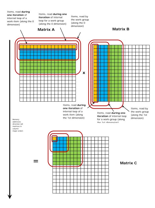
An "internal loop" is one of the loops by ib or jb (depending on dimension considered: 0 or 1 correspondingly) in the pseudo-code of the tiled matrix multiplication. Each work-item in this example processes one stridden 2x2 tile reading and writing with the following matrix elements:
