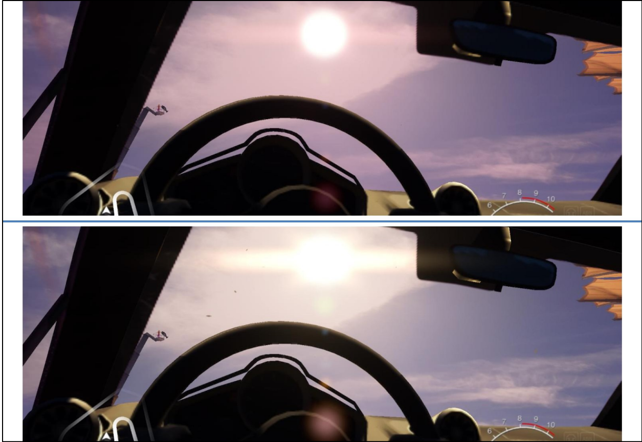
Figure 3: Screen shots of sunlight through the windshield before (top) and after (bottom) programmable blending is applied. Courtesy Kettlewell/Davies 2014 GDC presentation (see slides 27 and 28)
