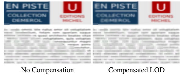
Figure 2: A zoomed-in image, rendered with smoothly varying CP parameters having a smaller value towards the top right and a larger value towards the bottom left. Quantizing the CP parameters can produce visible discontinuities in the CP size (top), which can be masked by compensating the LOD calculation in the texture sampler (bottom).
