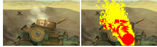
Figure 9: A simple culling example of soft particles (left). The right image shows the culling potential by discarding fully transparent regions (yellow) in the coarse pixel shader, and performing a coarse depth test (red).
