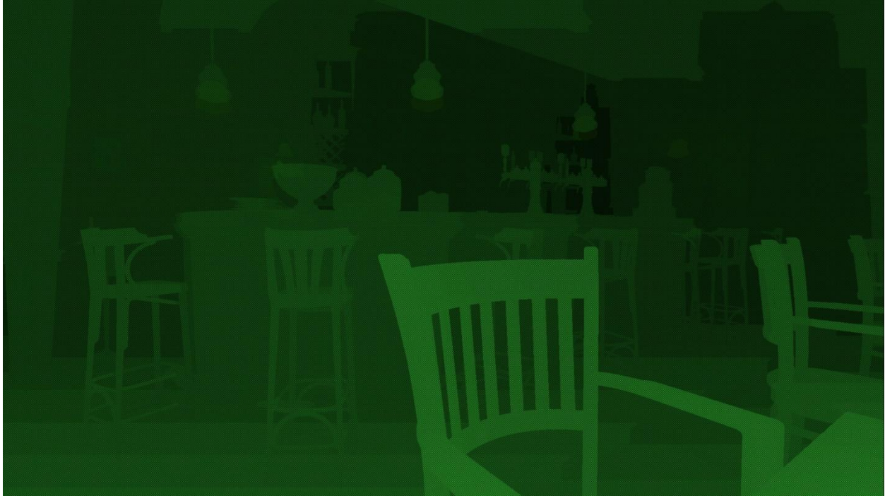
Figure 16: Per pixel motion vectors derived from the depth buffer. The camera is translating up (positive Y ), the magnitude of the Y motion per pixel is reflected in the green channel of the render target. In this scenario, foreground objects have larger motion vectors between frames.
