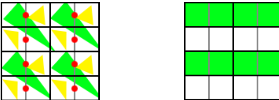
Figure 2: Shading information is lost due to sample coverage positions; the light-gray outlines represent the pixels of a full-resolution render target, the black outlines represent the pixels of a half-resolution render target. Left: Triangles to be rasterized to the render target, the red dots represent the sample coverage position for each half-resolution pixel; notice only the green triangles pass the coverage test. Right: The shaded pixel colors based on the results of the coverage test; the yellow triangles failed the coverage test and the render target cannot be accurately reconstructed during upscaling.
