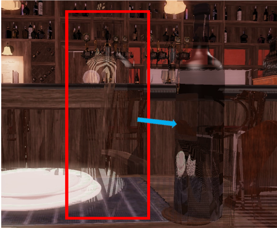
Figure 18: The red outline highlights the ghosted artifacts that appear when resolving the barstool. This is due to the required shading information being occluded by the wine bottle in frame N-1 .
