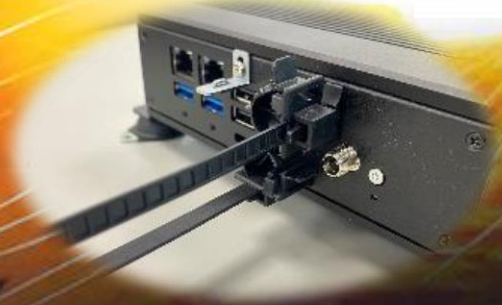
Lockable design reserved for I/O cables
