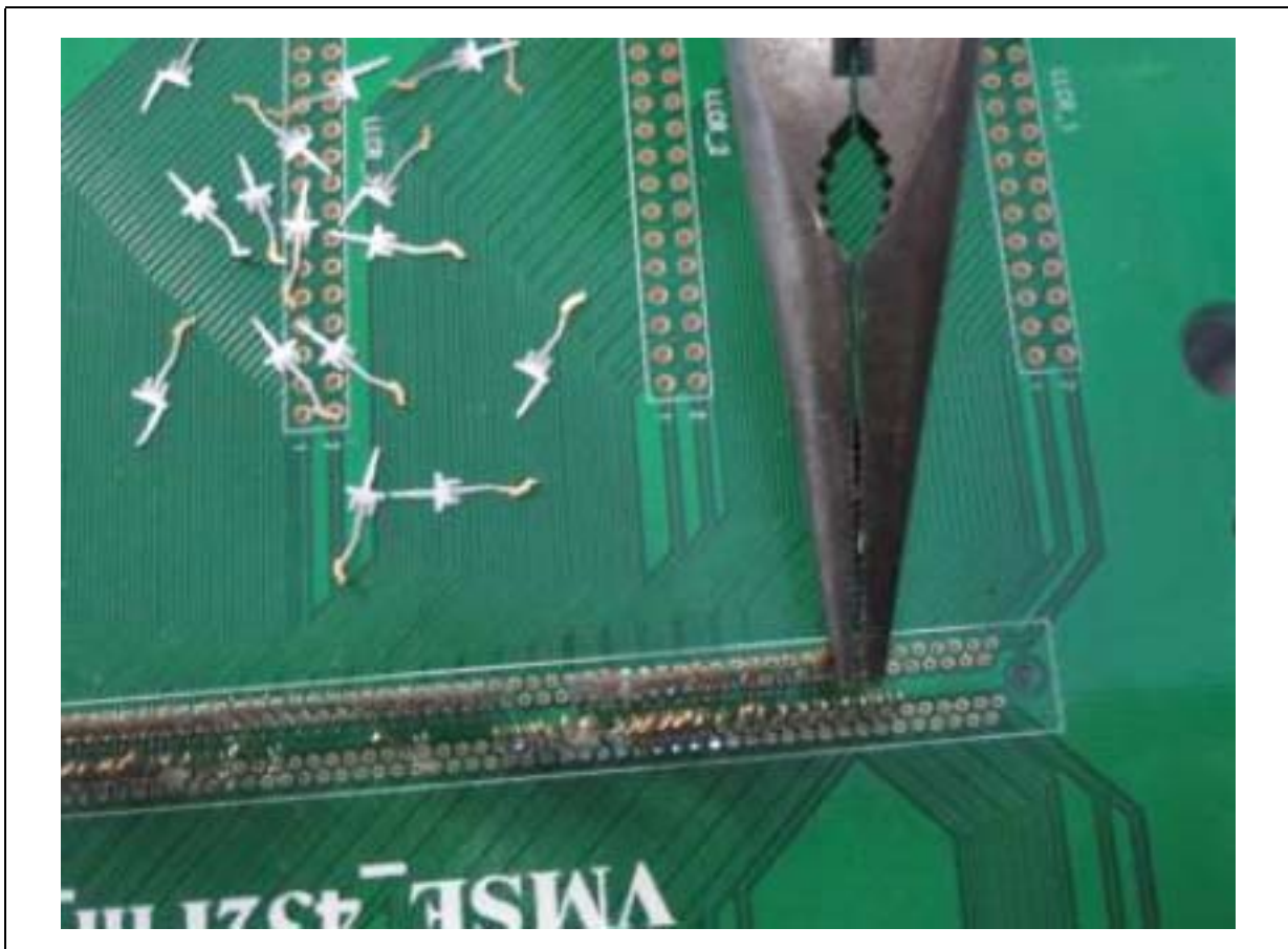
Figure D-6. Example of Manual Pin Removal
